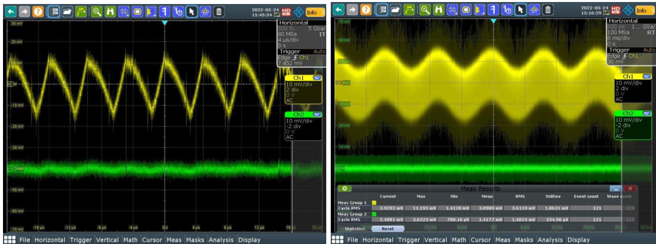
Figure 7: Switching ripple (left) and 100 Hz disturbance signal v_{out} and v_{FB} (right)
