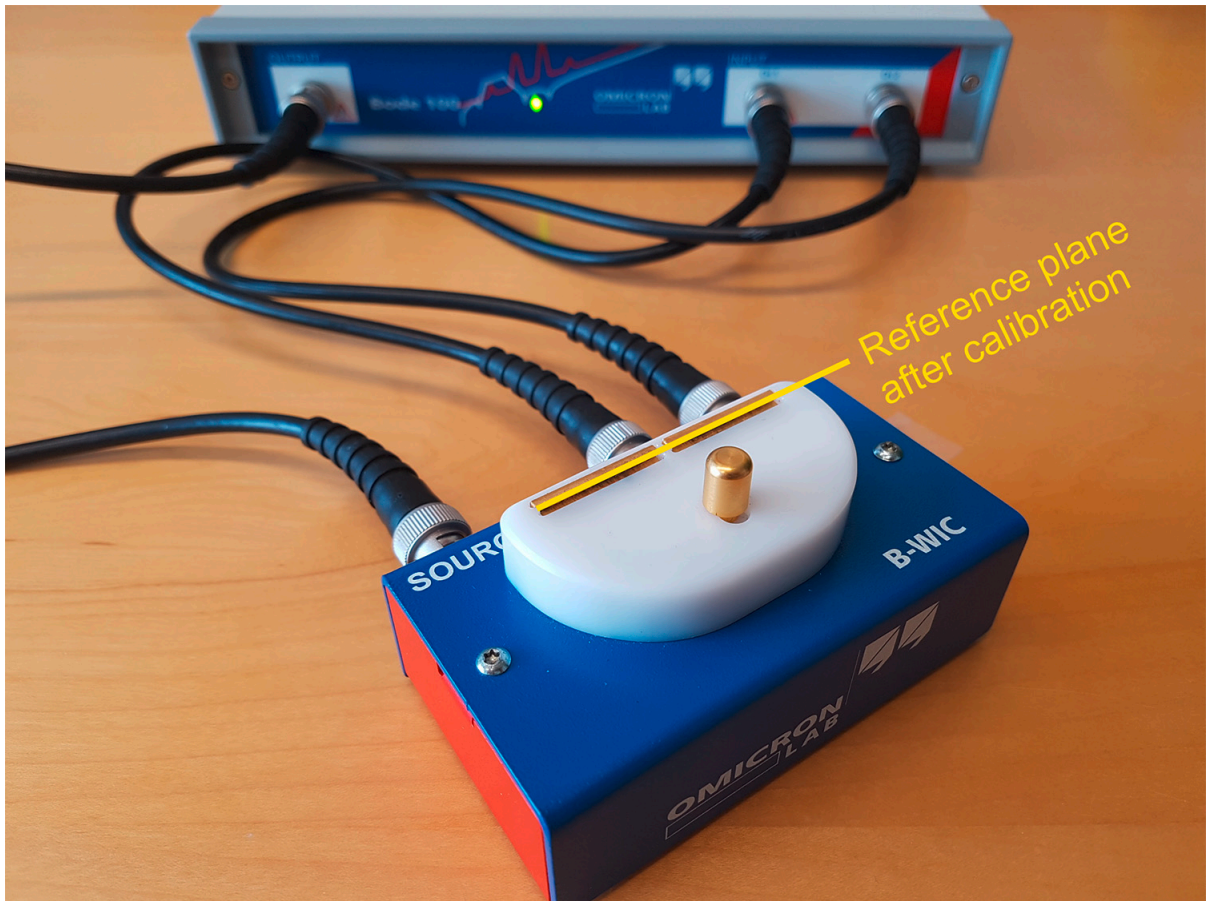
Figure 8-6: Calibrating the B-WIC impedance test fixture by performing Open, Short and Load Calibration
