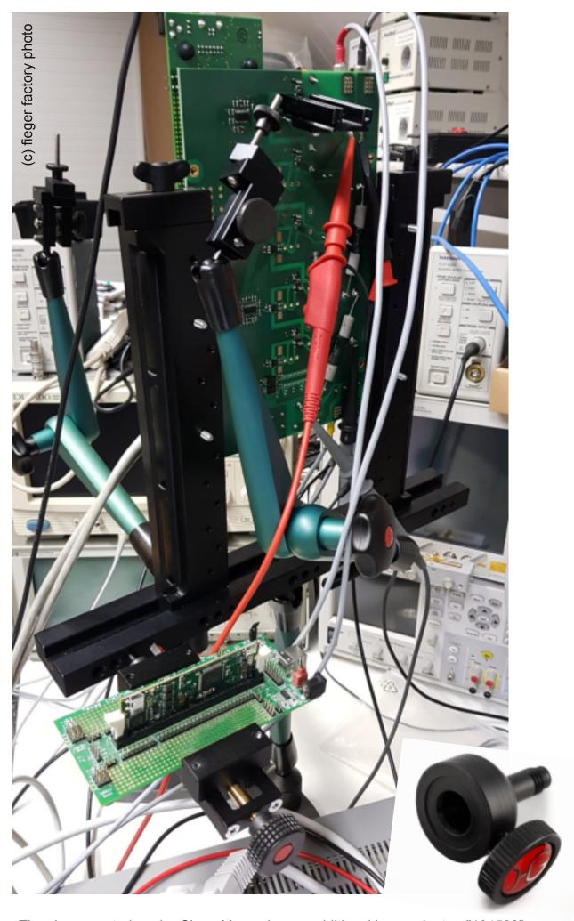
The vice mounted on the ClampMan using an additional base adapter "104500"
