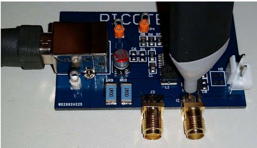
The 1-port probe is terminated into a P2130A DC Blocker and a 50 ohm scope input.
