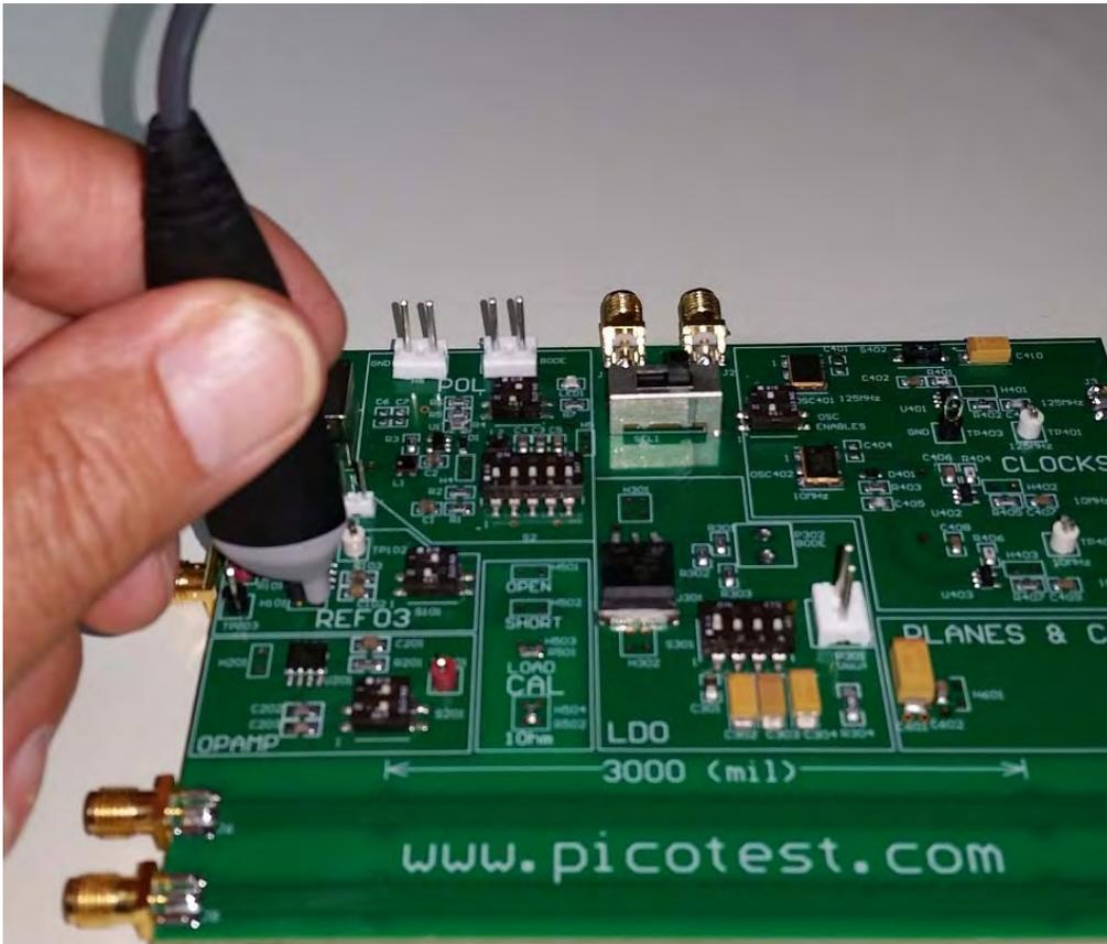
The 1-Port probe is used to make an output impedance measurement of a voltage reference.
