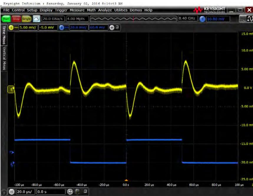
The transient step load response of the voltage regulator using the browsing capability of the 2-Port probe.
