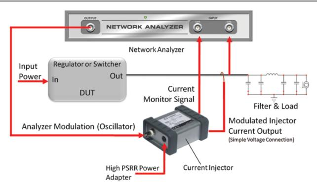
The J2112A Current Injector supports non-invasive phase margin measurements. You can actually use it to measure the stability of your power supplies WITHOUT having to break the control loop. Simply connect the Current Injector output (+ and – leads) to the signal of interest and you can measure the impedance, stability, or step load response.
