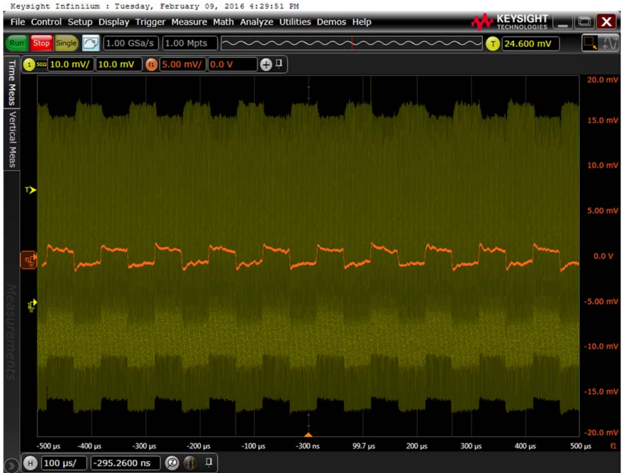
Figure 3 Load Step J2150A mode 5 orange trace is averaged 500ohm scope input with P2130A 500Hz-8GHz DC block
