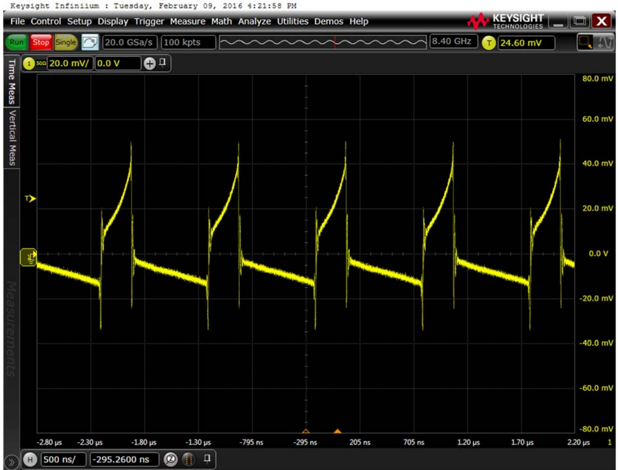
Figure 5 Full bandwidth, 50Ohm scope input with P2130A 500Hz-8GHz DC block
