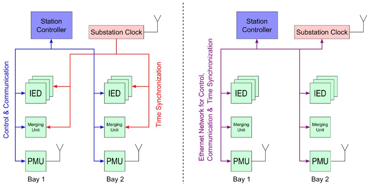
**Figure 2 - Time distribution infrastructures in substations**
