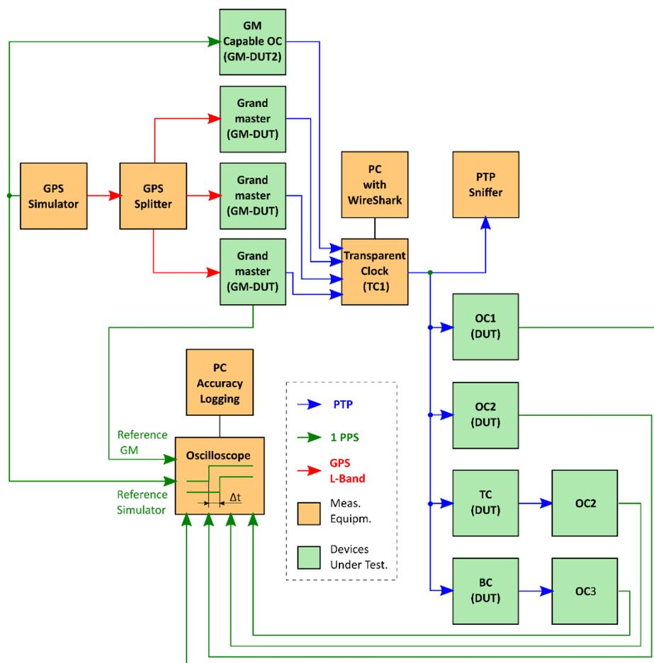
Figure 9 – Example for a test setup used during the IOP 2015
