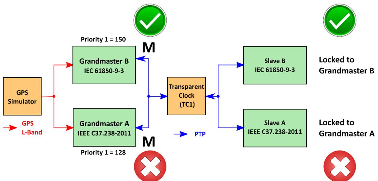
Figure 13 – BMCA test with IEC 61850-9-3 as the best clock
