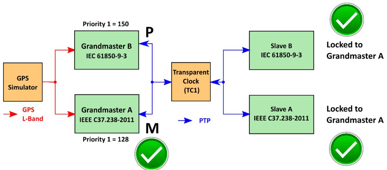
Figure 12 – BMCA test with IEEE C37.238 as the best clock
