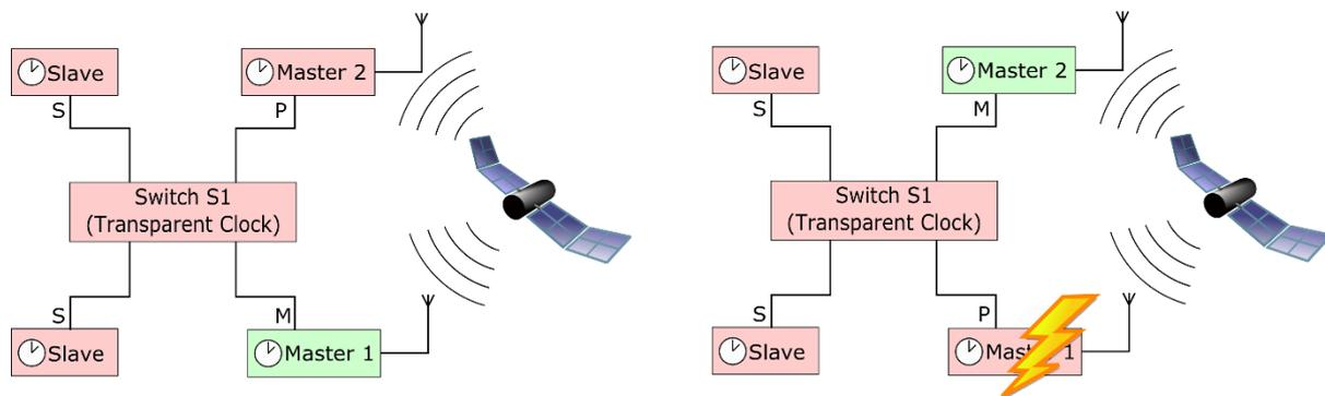
**Figure 6 – Concept of BMCA switch over**
