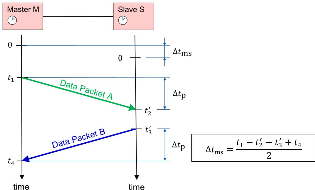
Figure 3 – Determination of the time offset  $\Delta t_{ms}$  between master and slave
