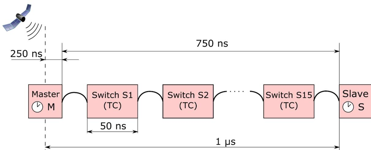
**Figure 8 – Time inaccuracy for a chain of transparent clocks**
