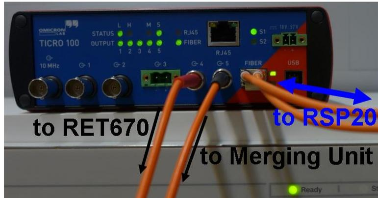
Figure 2: Connecting RET670 with TICRO 100
