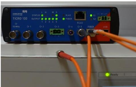
Figure 14: red IRIG-B ST Fiber disconnected
