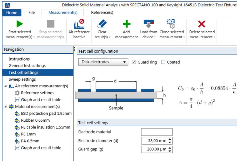
Figure 5: Test cell settings to be selected for Dielectric Test Fixture 16451B - Electrode A
