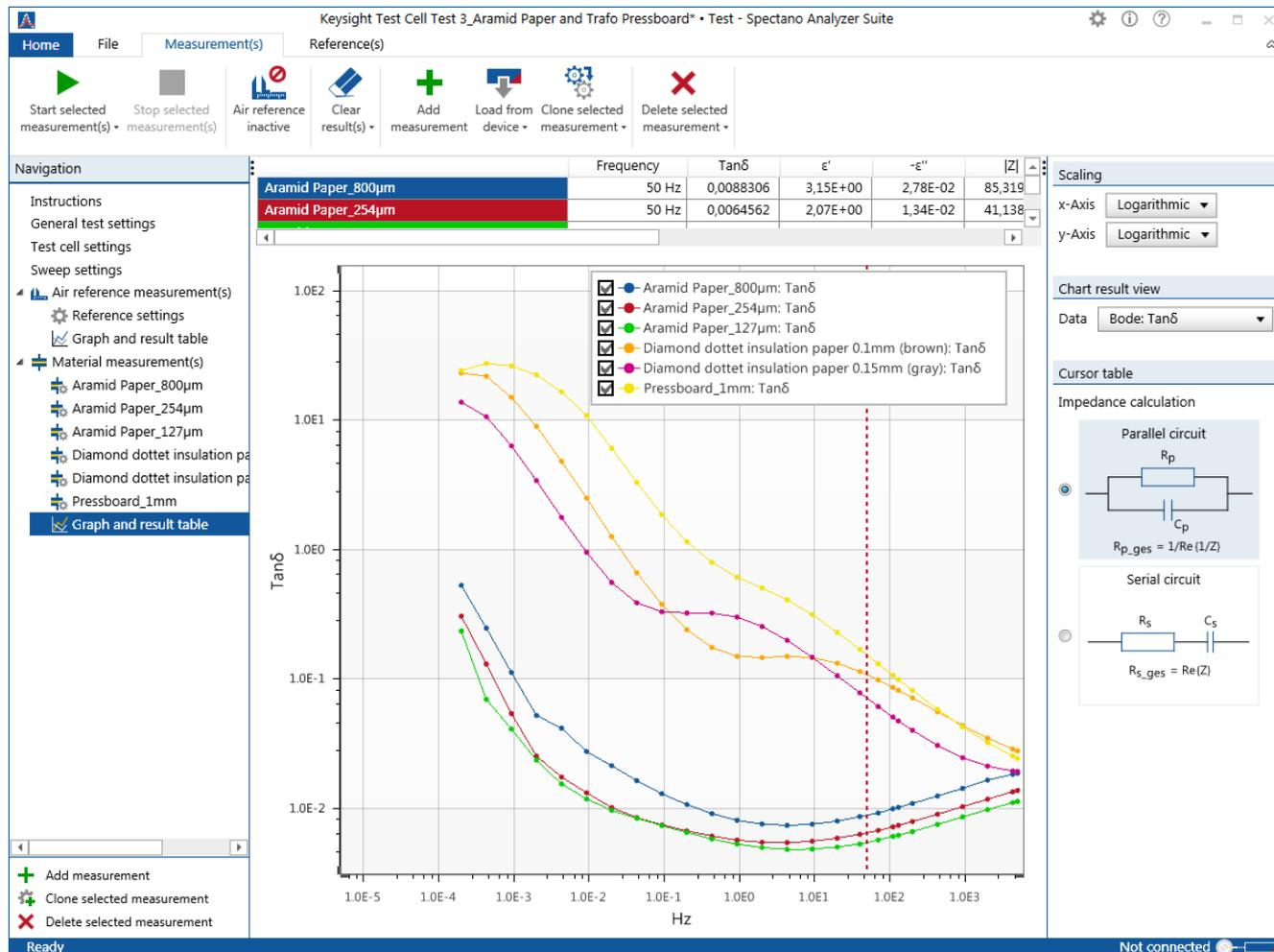
Figure 14:  $\tan(\delta)$  example curves of different aramid and insulation papers
