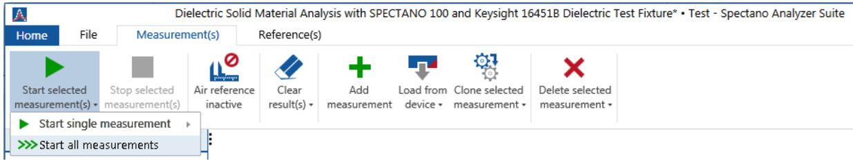
Figure 9: Start measurement sequence
