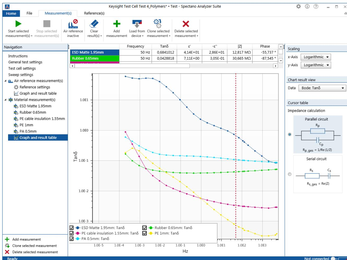
Figure 12:  $\tan(\delta)$  example curves of different polymers
