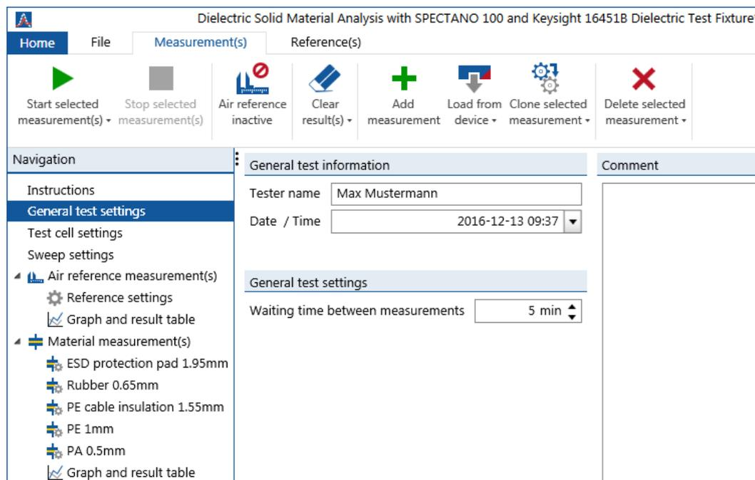
Figure 4: General test settings example for measurement of different polymers and plastics
