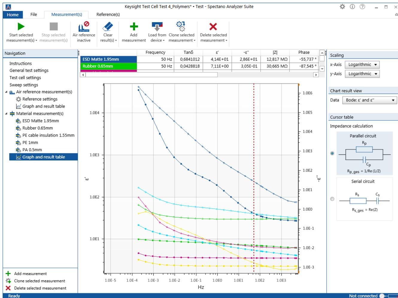
Figure 13: Relative permittivity example curves of different polymers
