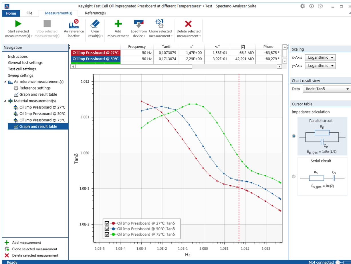
Figure 15:  $\tan(\delta)$  example curves of oil impregnated paper
