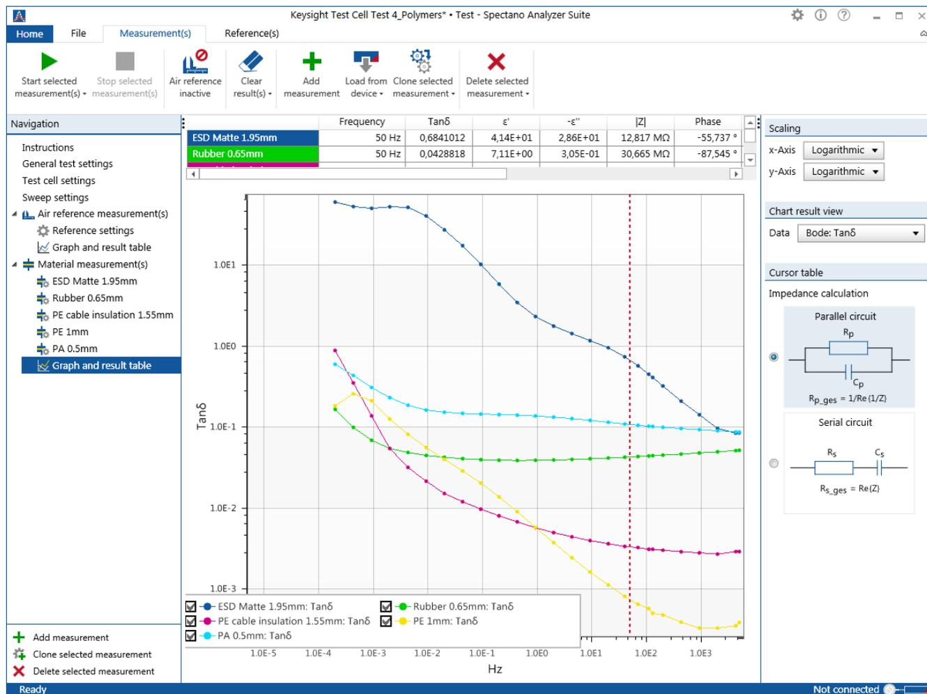
Figure 12: Tan(δ) example curves of different polymers
