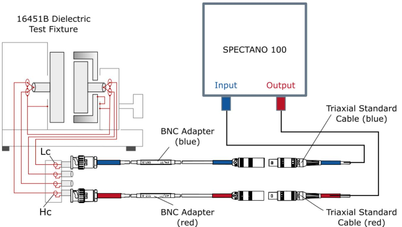
Figure 2: Setup schema using SPECTANO 100 and Dielectric Test Fixture 16451B from Keysight
