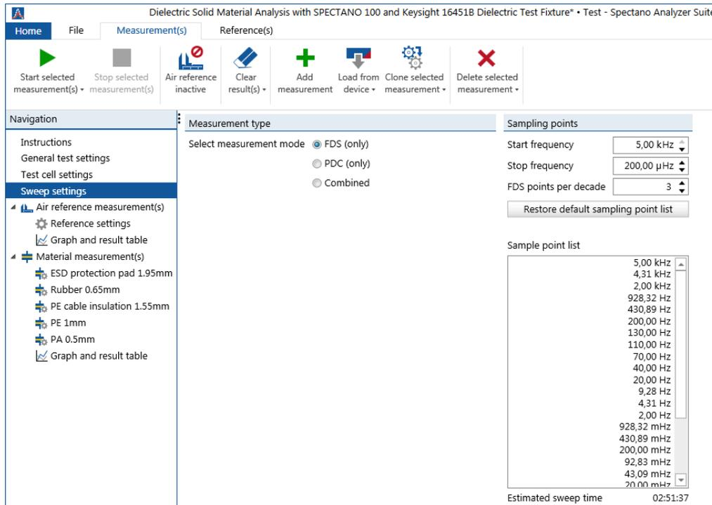
Figure 6: Sweep settings example for measurement of different polymers and plastics
