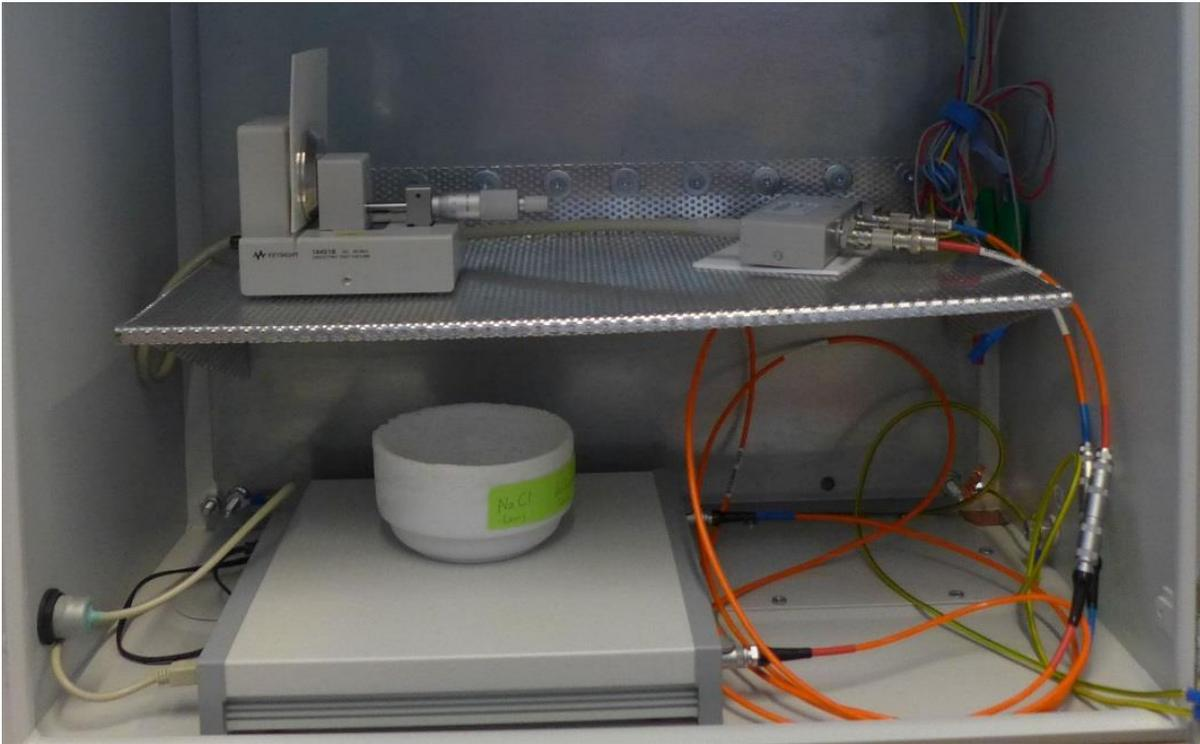
Figure 1: Dielectric material analysis using Dielectric Test Fixture 16451B from Keysight - Setup
