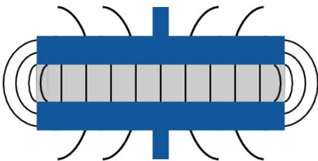
Figure 3: Lines of electric force, unguarded electrode<sup>2</sup>
