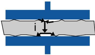
Figure 2: Bad contact between material sample surface and electrodes<sup>1</sup>
