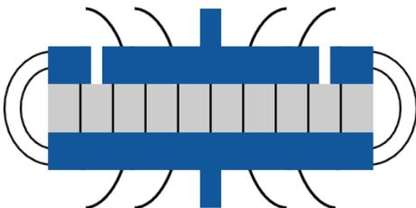
Figure 4: Lines of electric force, guarded electrode<sup>3</sup>
