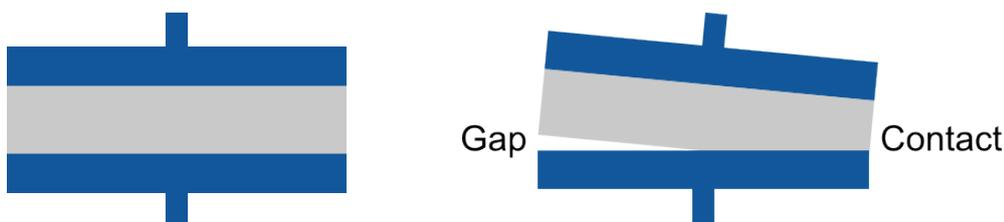
Figure 1: Correct (left picture) and wrong (right picture) adjustment of the test cell
