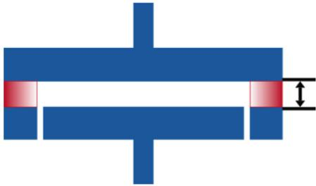
Figure 7: Adjusting the air gap height by using a spacer
