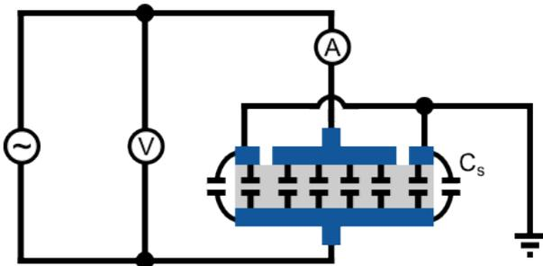
Figure 5: Measurement circuit, guarded electrode ( $C_s$  is stray capacitance)
