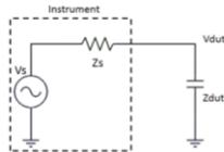
Figure 1. Schematic of Capacitance Measurement with Source Impedance
