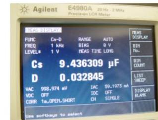
Figure 4. Capacitance measurement of 10 μF capacitor using ALC function.
