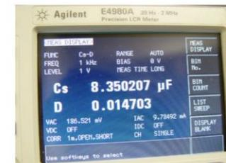
Figure 3. Capacitance measurement of 10 μF capacitor.
