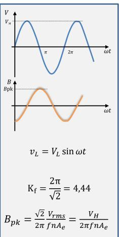
K<sub>f</sub>: waveform coefficient
