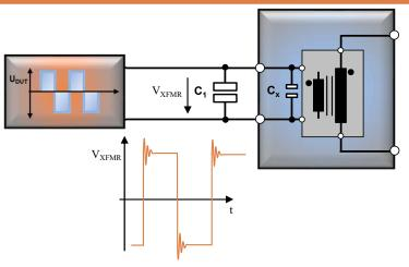
$f_{x} = \frac{1}{2\pi\sqrt{LC_{x}}}$   $f_{1} = \frac{1}{2\pi\sqrt{L(C_{x} + C_{1})}}$   $C_{x} = \frac{C_{1}}{\left(\frac{f_{x}}{f_{1}}\right)^{2} - 1}$
