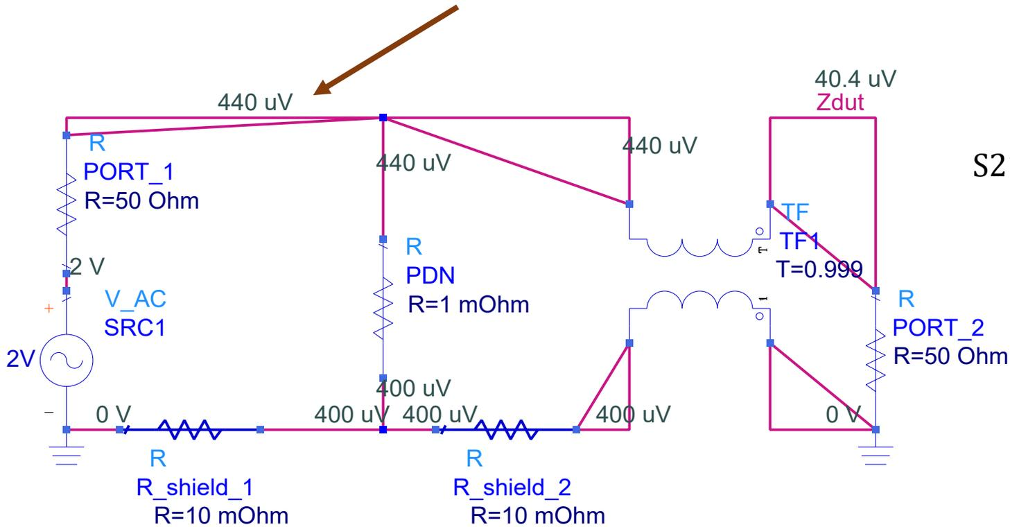
Here the ground is isolated by the CMRR of the isolator
