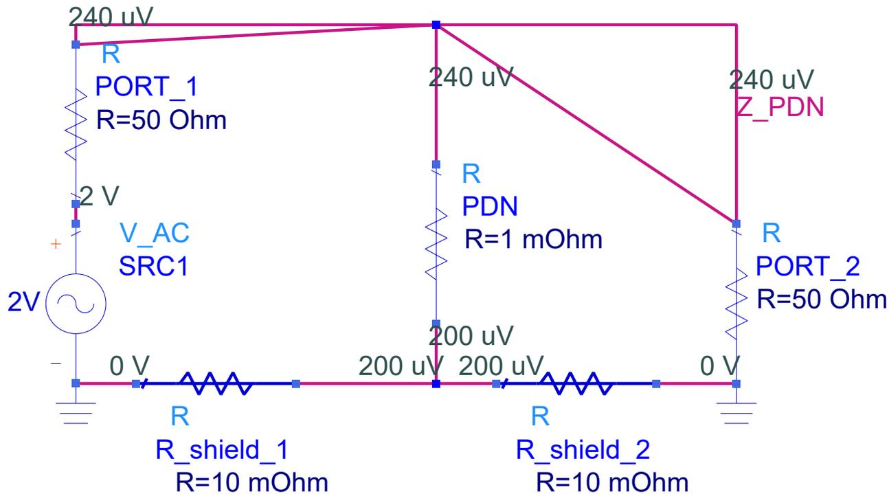
$$S_{21} \approx \frac{\frac{R_{\text{shield}_1} \cdot R_{\text{shield}_2}}{R_{\text{shield}_1} + R_{\text{shield}_2}} + DUT}{25 + \frac{R_{\text{shield}_1} \cdot R_{\text{shield}_2}}{R_{\text{shield}_1} + R_{\text{shield}_2}} + DUT} = 240u = -72.4dB$$
