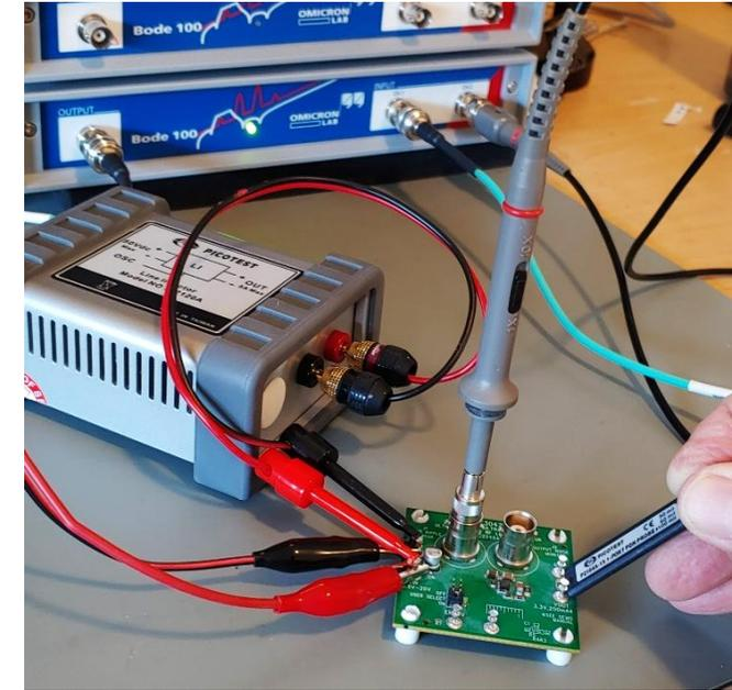
The power supply modulation setup is the same for PSRR, PSMR, and PSNR
