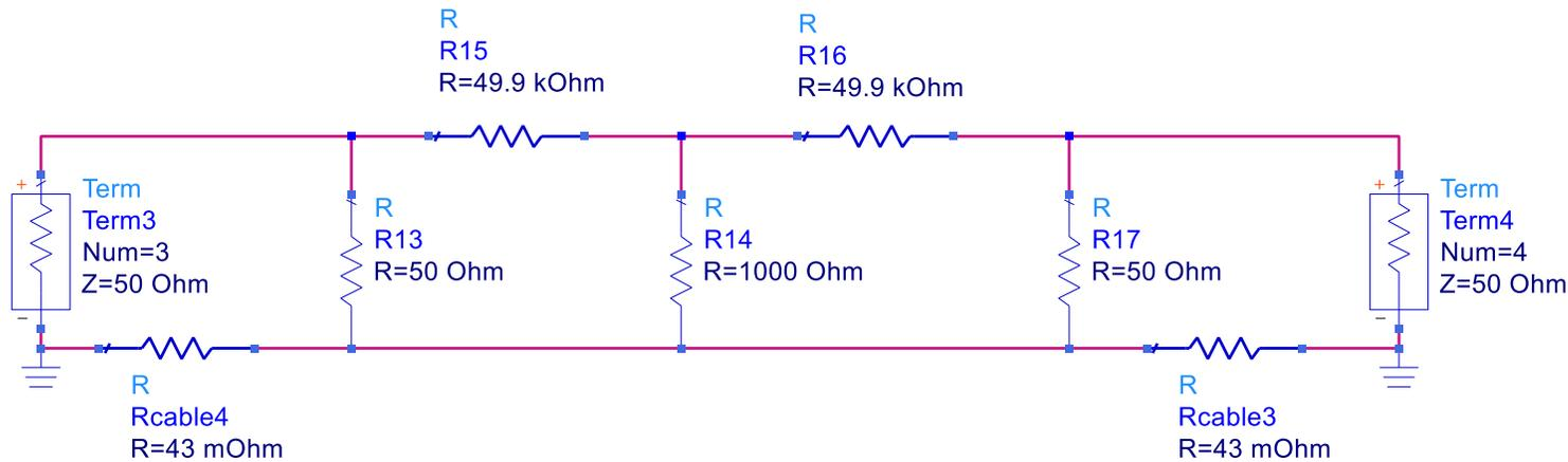
Include the cable shield resistance
