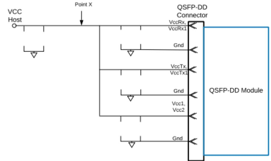
Figure 11: Module Noise Output Measurement
