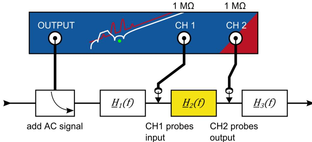
Note: Use the external reference function of the Bode 100 to enable CH1 input!
