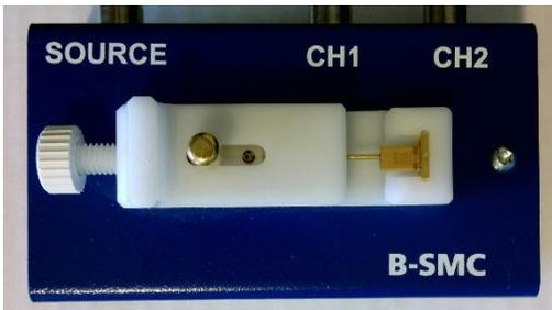
An impedance fixture can be used if  $\text{ESR} \geq 100\text{m}\Omega$
