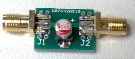
Low ESR caps must be mounted in a calibrated PCB for measurement
