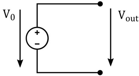
$$R_{out} = 0 \rightarrow V_{out} = V_0$$
