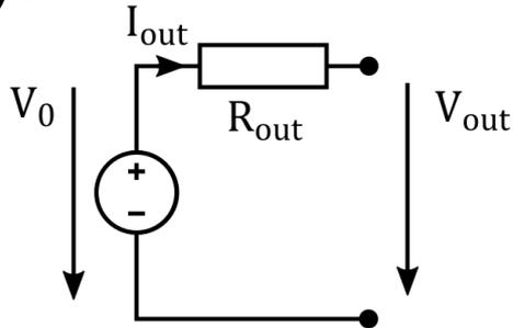
$$R_{out} \neq 0 \rightarrow V_{out} = V_0 - I_{out}R_{out}$$
