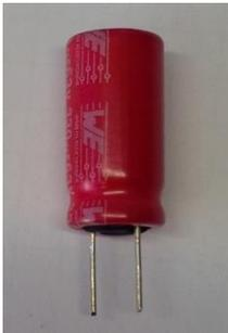
$$\text{Capacitor: } i(t) = C \frac{dv(t)}{dt} \quad X_C = \frac{-1}{\omega C} \quad \frac{V}{I} = Z_C = \frac{1}{j\omega C}$$
