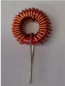
$$\text{Inductor: } v(t) = L \frac{di(t)}{dt} \quad X_L = \omega L \quad \frac{V}{I} = Z_L = j\omega L$$
