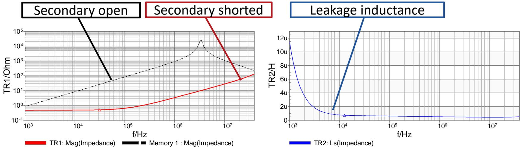
→ Leakage inductance is not constant over frequency
