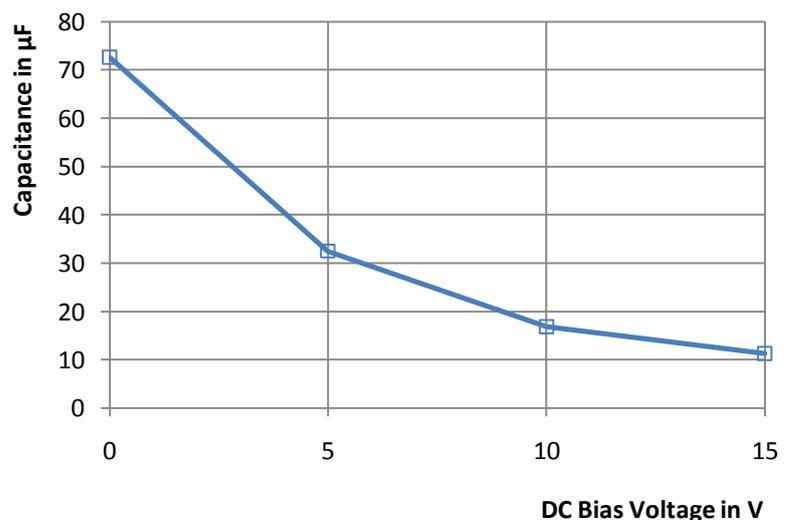
From the measured results we see that the capacitance strongly decreases with increasing DC Bias voltage. Furthermore the capacitance does not reach the nominal value of 100  $\mu$ F at 0 V DC bias.
